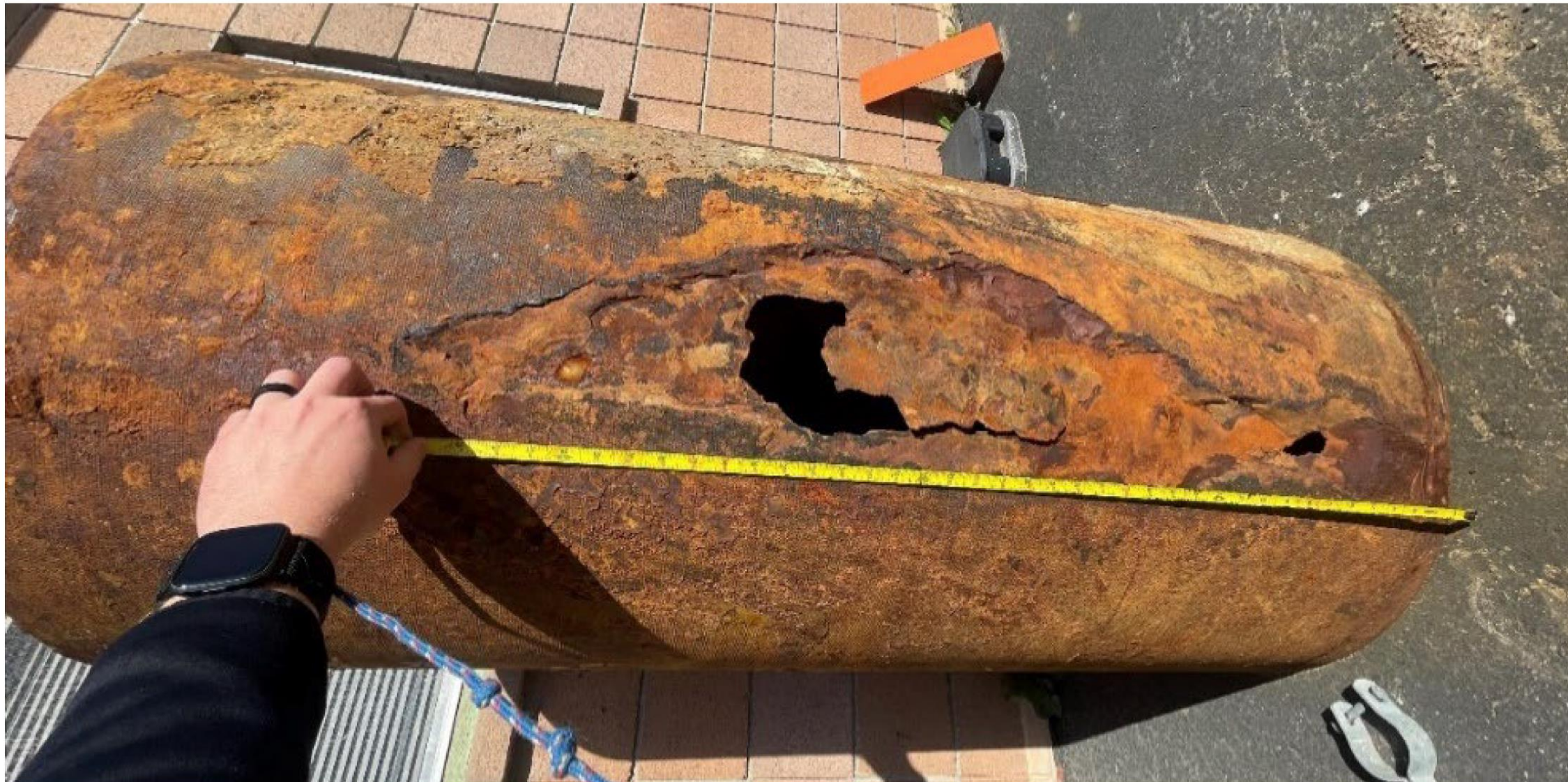
Figure 7: Failure section of the pipe
